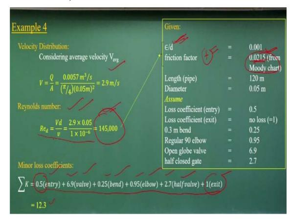
Since here the roughness factor is given to us, we need to compute the friction factors from Moody's chart which needs Reynolds numbers. So first let us compute what will be the average velocity and what could be the Reynolds numbers for this flow. Diameter is given, velocities, then we can get this. So these Reynolds numbers with these roughness factors we will get it from Moody's charts, the value of friction factor.
