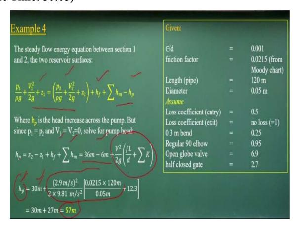
Now we will go to the next what we will do it is very simple things that we are applying this energy equations head loss and this part since two part  $V_1$ ,  $V_2$ , if I put the energy losses  $V_1$ ,  $V_2$  is zero, and solving this pumping head, okay which is will give it the elevation difference and the major and the minor losses component. Then I will get it what is the head requirement at the pump which is coming out to be 57 meter, okay.
