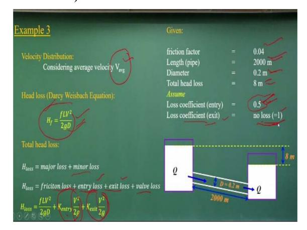
So the friction factors data what is given it length of the pipe the diameters and total head losses. The loss coefficient in terms of velocity head as you know it at the exit we consider as 1, at the entry we consider 0.5. The half of the velocity head losses at entry levels and at the exit level total velocity head what we lost it at the exit level. This is 1, this is 1.5.
