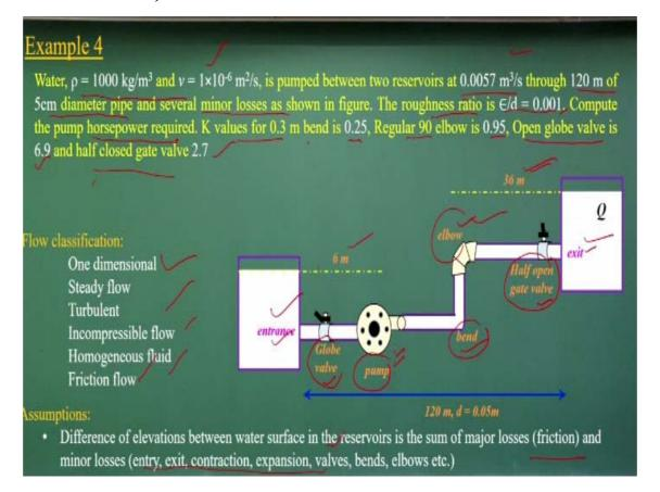
The last examples, let us have a it is slight bit a design problems could be consider it where you have the two reservoirs okay you have a entrance and exit. The water density and the kinematic viscosity is given to us. The two reservoirs having the discharge 120 meter long, 5 centimeter diameter pipe several minor losses can happen it like a valve losses.
